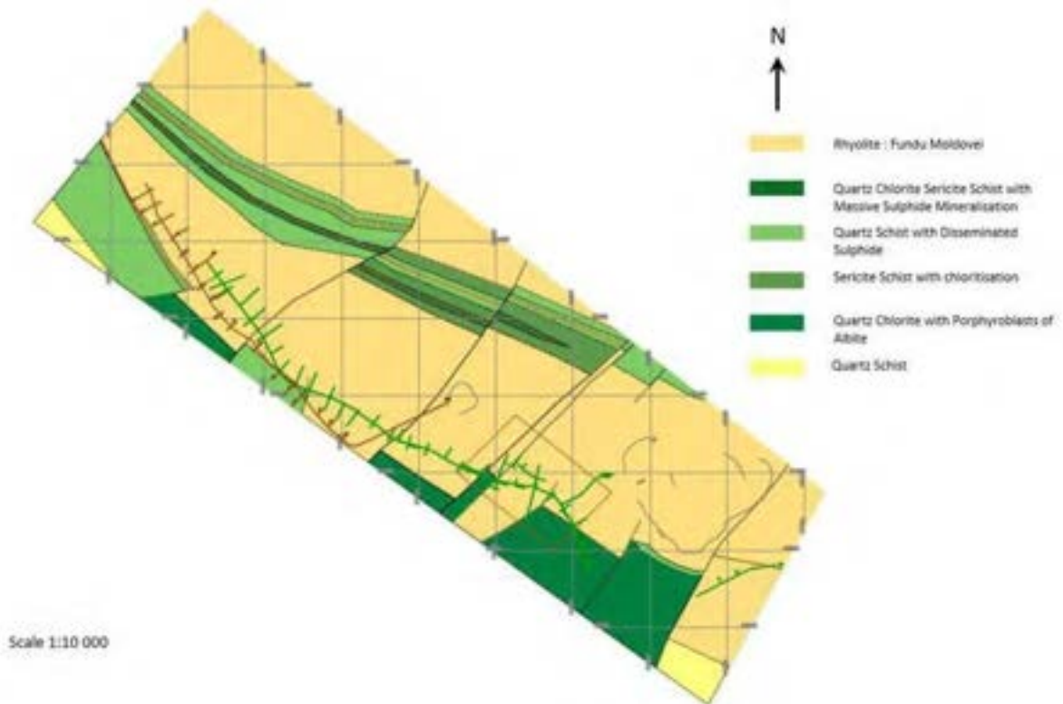
Figure 6-10: Detailed surface geology of the Manaila deposit. From: Harvey (2018).
